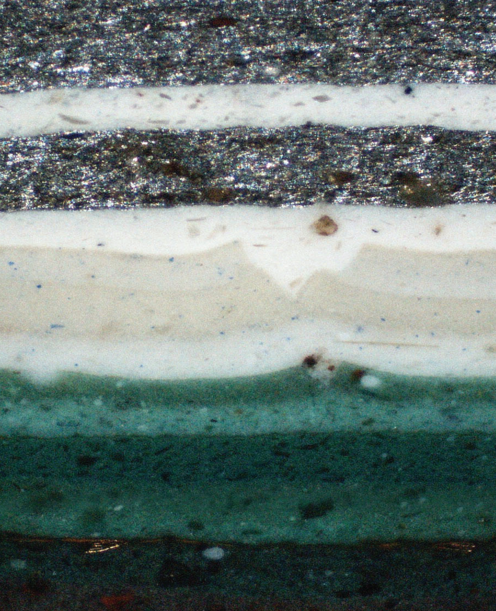
Photomicrograph of cast iron porch railing.
